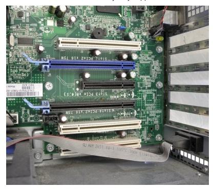
5. Insert the SafeNet Luna PCIe HSM card into the connector. It should go straight in – angling the card might cause it to bend. The card is properly seated when no portion of the gold-colored contacts of the card protrudes above the connector socket.
