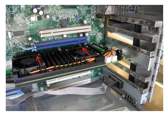
6. Secure the card hold-down bracket with a screw.
